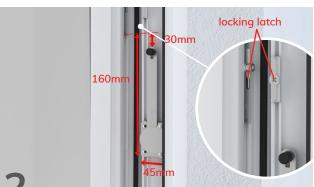
Insert the blockade into the window frame at a distance of about 160 mm from the locking latch (it is important that to position the blocking arm to be approx. 30 mm under the locking bolt).
